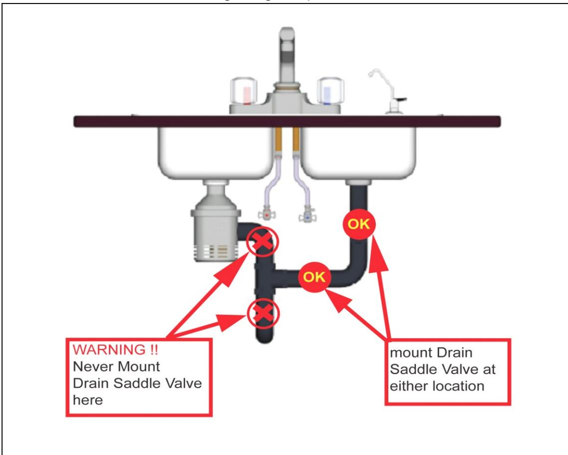
1. Choose a spot on the drain pipe that is convenient for installing the drain saddle. A horizontal pipe is recommended to minimize the dripping sound.
