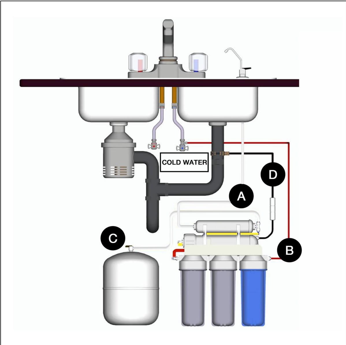
Please follow the color-coded tube connections to complete the installation.
