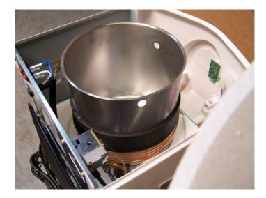
11.7 Disconnect (2) wires from sensor switch
