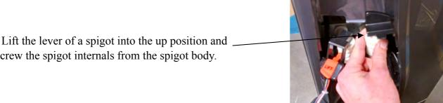
1.4 Lift the lever of a spigot into the up position and \_ unscrew the spigot internals from the spigot body.
