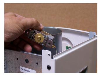
11.10 To remove the sensor tube, carefully pull the sensor out of the copper tube at the bottom outside of the cold tank
