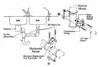
Drain saddle connection method
