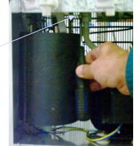
5.11 Remove (1) hot tank screw from below
