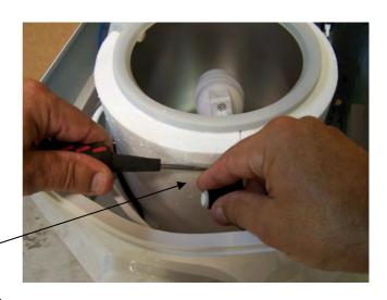
4.2 Remove elbow connector from float stem
