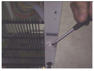
9.1 Remove the plug with fingers. Water will pour from the port
