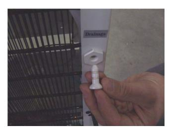
9.2 Drain any remaining water in the system by depressing the faucets.
