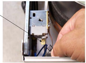
11.8 Remove (2) screws holding sensor switch body to cooler cabinet.
