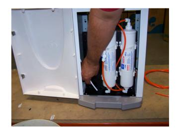
2.6 Remove outlet line of carbon filter (bottom)
