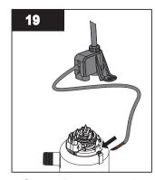
Connect the green ground wire and red strain relief wire to the chamber using the grounding screw.
