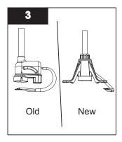
For older style Lamp Connector follow steps 4 and 5. For new Lamp Connector follow steps 6 and 7.
