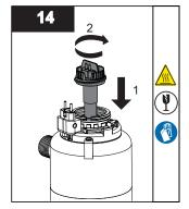
Insert new lamp into the quartz sleeve and thread into sleeve bolt until hard stop.
