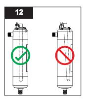
Ensure quartz sleeve is properly centered in the chamber.
