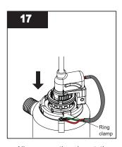
Align connections by rotating ring clamp to push lamp plug onto end of lamp.
