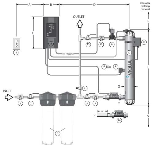
Figure 2 System - Dimension and Layout
