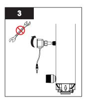
Install the sensor to the UV system (for PRO models only).
