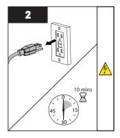
Disconnect main power source and allow the unit to power down for 10 minutes.
