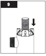
Reinstall the sleeve with arrow pointing up.
