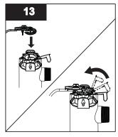
Install lamp harness onto chamber.
