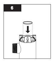
• Wet O-ring with water then place over top end of sleeve.
