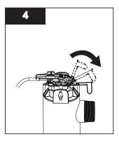
• Pinch wire form to release the lamp connector.
