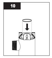
Reinstall the new lubricated O-rings over the top end of the sleeve.
