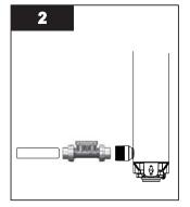
Connect Flow Meter Sensor (PRO10,20,30 models only) to chamber using 11/4" unions supplied.
