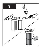
With all faucets closed, remove filter housing(s) using sump wrench.
