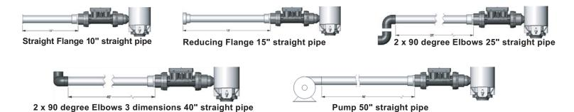
**Note:** Flow Meter Sensor must be mounted in the following orientation with the LED facing up. Ensure all air is purged from the piping and Flow Meter Sensor. All straight length to the Flow Meter Sensor must be 1.00" in diameter.
