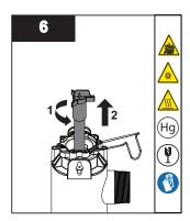
• Rotate and remove the UV lamp from the sleeve.
