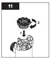
Connect the sleeve bolt to the top of the sleeve assembly.
