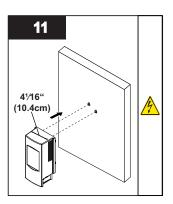
Install the controller unit to the wall. Ensure that the controller is installed higher than the chamber and away from all water sources.
