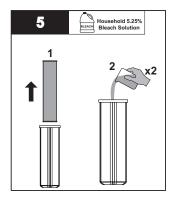
Remove cartridge(s) and pour 2 cups of household bleach solution into the filter housing(s).
