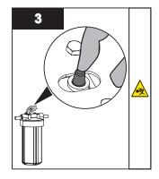
Press the pressure button to release the pressure from the cartridges.
