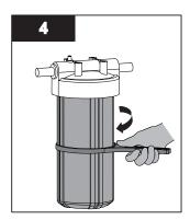
Remove filter housing(s) using sump wrench.
