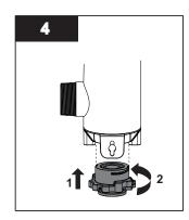
Connect the sleeve bolt at the bottom of the sleeve assembly. Ensure sleeve bolt is rotated full 1/4 turn until positive stop.
