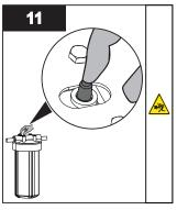
Press the pressure button to purge air and to complete the disinfection procedure.
