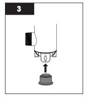
• Insert the sleeve removal tool into the bottom of the sleeve.
