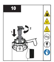
Install and rotate the lamp into the sleeve assembly.
