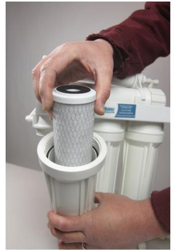
5. Tighten the center sump hand tight and secure it with the supplied filter wrench by turning it an additional 1/4 - 1/2 turn.
