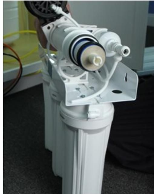
2. Use the supplied wrench to remove the membrane housing cap.
